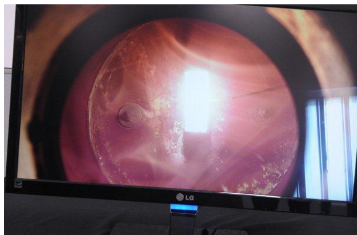
Nanoparticles are produced and harvested Monday in a reactor at Nanomech. Copper wire is fed into the reactor to make the nanoparticles that appear as wispy smoke in the reactor. Photo by J.T. Wampler
