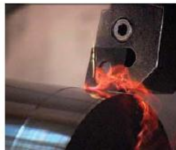
A CBN-coated tool in a turning operation.
